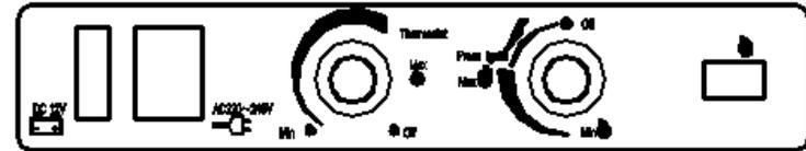
DC Connector AC Connector Thermostat Knob Gas Regular Knob Gas Meter
