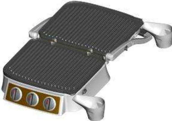
For using the griddle you have to open the grill totally by pushing on the safety button at the side (10). Then you can open the grill totally and the upper flat plate (8) can rest on the handle (2). Keep in mind that your grill has a grill plate (6) and a flat plate (8). You can see on the picture how to use the drip cups (11). The griddle knob (3) can be changed into different temperatures.
