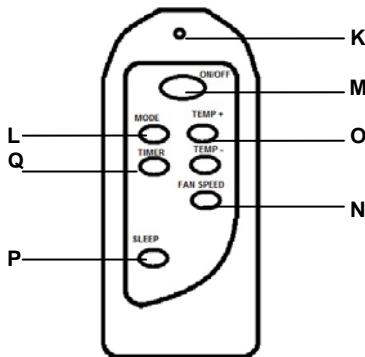
**K** Control light, lights up when the keys are operated.
