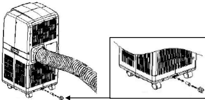
If the condensation must be removed continuously, place the condensation drain hose (No. 16) on the spout. Do remove the rubber plug. The condensate drain hose can be extended with another hose (not supplied). It can be connected to a drain or be led outside. Make sure this hose does not go up.
