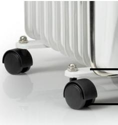
Place the pins of the castor wheels in the 4 holes of the metal wheel plates and fix them with the nuts. Turn the radiator back to its correct upright position.
