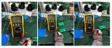
2, mos-tube: the multimeter-to-diode-gear (mos-tube-belongs-to-semiconductor-components, withthis-gear-measurement-is-more-accurate), with-positive-and-negative-table-pen-measuring-mos tubegd, ds, when one end data-is zero, one end data-(figure 2), the mos-intact, when both-have data-(figure-1), the mos tube-is-breakdown, need-to-be-replaced-newe
