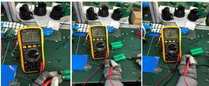
2. mos tube: the multimeter to diode gear (mos tube belongs to semiconductor components, with this gear measurement is more accurate), with positive and negative table pen measuring mos tube  $gd_s$ , when one end data is zero, one end data (figure 2), the mos intact, when both have data (figure 1), the mos tube is breakdown, need to be replaced new
